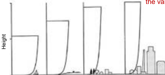
A: Open sea B: Open level, country C: Suburbs, woodland D: City centres Smooth → Rough
