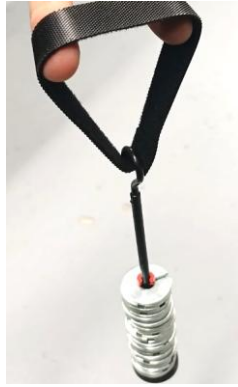
Figure 2 Fastener for hanger load
